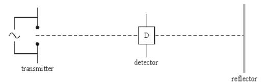
(i) Explain why the strength of the detector signal varied repeatedly between a minimum and a maximum as the detector was moved slowly away from the transmitter along the dotted line.
