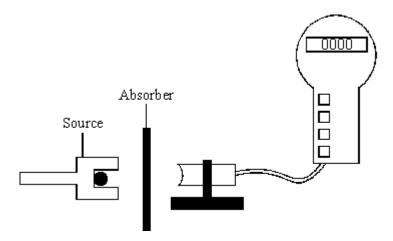
Two different types of absorber are placed one at a time between the detector and the source. For each absorber, a count is taken over ten minutes and the average number of counts per second worked out. The results are shown in the table.
