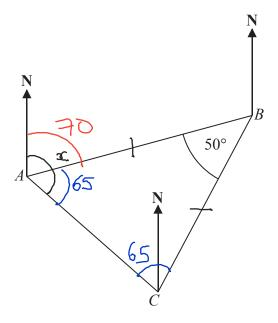
The bearing of B from A is  $070^{\circ}$
