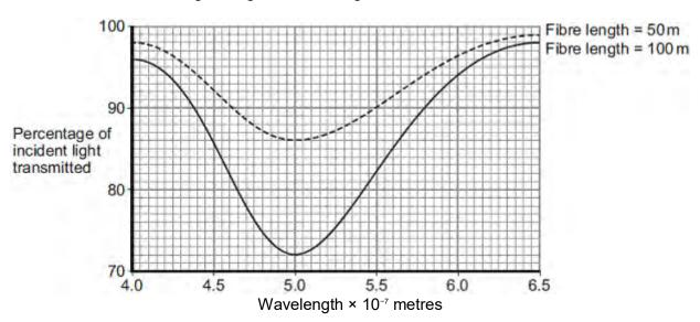
Compare the percentages of incident light transmitted through the two different fibres over the range of wavelengths shown.
