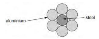
The resistance of a length of 1.0 km of the steel wire is 3.3  $\Omega$ . The resistance of a length of 1.0 km of **one** of the aluminium wires is 1.1  $\Omega$ .
