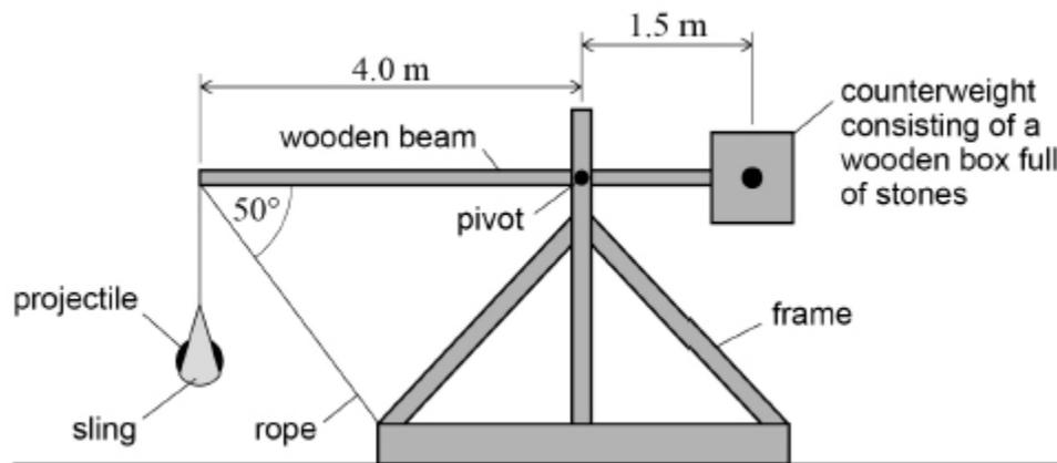
The counterweight is a wooden box full of stones attached to one end of the beam. The projectile, usually a large rock, is in a sling hanging vertically from the other end of the beam. The weight of the sling is negligible.
