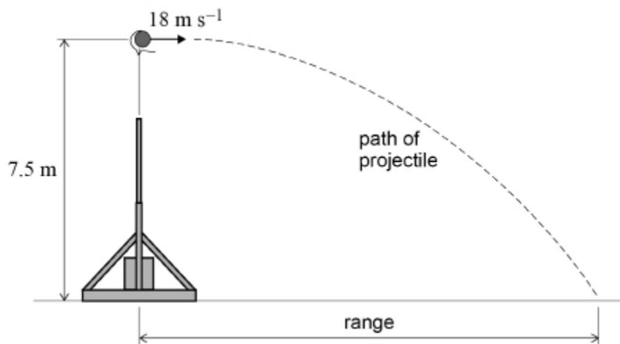
The range of the catapult is the horizontal distance between the point where the projectile is released to the point where it lands.
