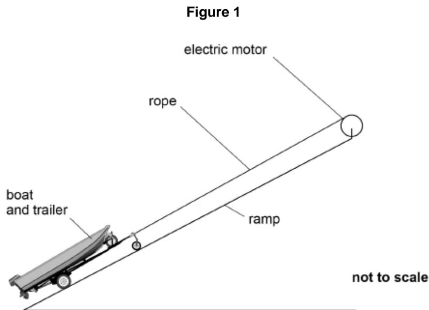
The boat and trailer are pulled by a motor which is connected to a 24 V battery of negligible internal resistance.
