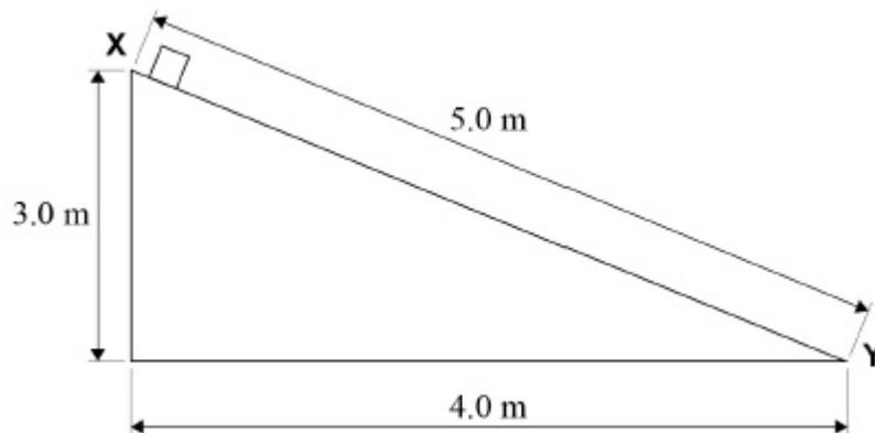
When the mass reaches **Y** at the bottom of the ramp it has a velocity of  $5.0 \text{ m s}^{-1}$ .
