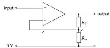
Two resistor chain, correctly labelled connected between output and ground
