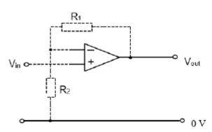
Correct configuration of  $R_1$  and  $R_2$   $\checkmark$
