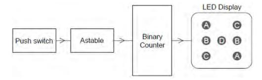
The binary counter consists of three rising edge triggered D-type flip-flops. The counter outputs are X, Y and Z. The most significant bit is Z.
