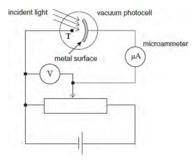
(a) The potential of the metal surface may be changed by adjusting the potential divider.
