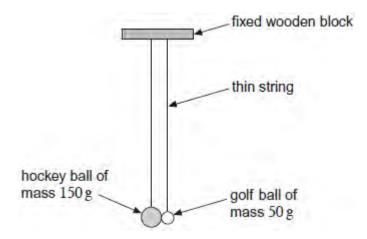
A golf ball of mass 50 g is initially hanging vertically and just touching a hockey ball of mass 150 g. The golf ball is pulled up to the side and released. It has a speed of  $1.3~{\rm m~s^{-1}}$  when it collides head-on with the hockey ball. After the collision the balls move in opposite directions with equal speeds of  $0.65~{\rm m~s^{-1}}$ .
