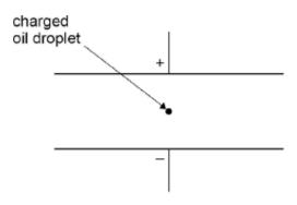
(a) The droplet falls vertically at its terminal speed when the potential difference (pd) between the plates is zero.
