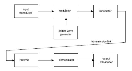
transmitter & receiver, carrier wave gen ✓ demodulator & modulator ✓
