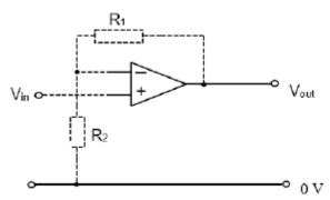
Correct configuration of  $R_1$  and  $R_2$   $\checkmark$
