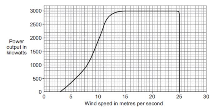
In one 4-hour period, the wind turbine transfers 5600 kilowatt-hours of electrical energy.
